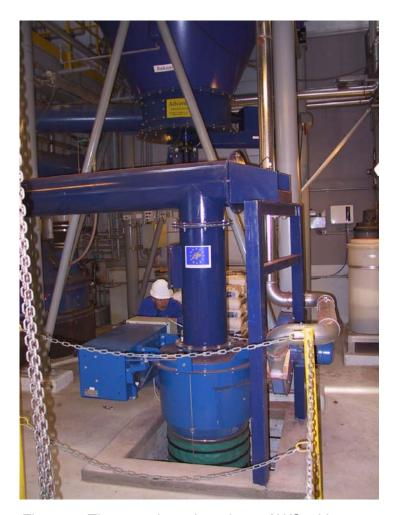
Figure 2. The new dry ash outlet at AWS with screw conveyor and load bellows.
