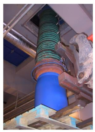
AWS 060530. Filling a 220 liter drum with dry bio ash.
