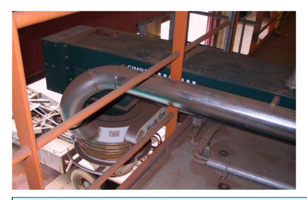
LYNIS 060622. The end of the new screw conveyor, the load bellows and the connecting tube to the air suction ventilator.
